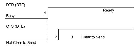
**1:** The application raises its DTR signal to indicate a ready state (meaning DTE wants to communicate with the DCE).
