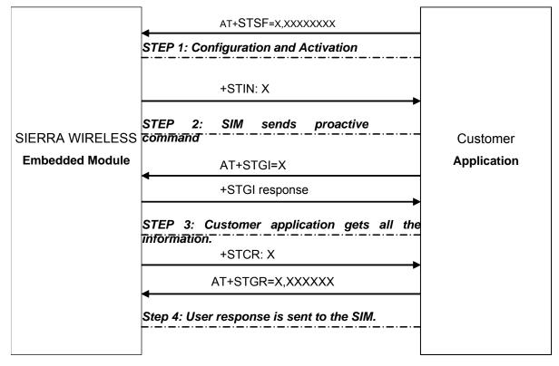
On the first step, the customer application informs the Sierra Wireless product which facilities are supported. This operation is performed with the +STSF (SIM ToolKit Set Facilities) command, which also allows to activate or deactivate the SIM ToolKit functionality.
