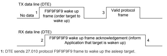
2: DCE replies with 27.010 F9F9F9F9 wake up frame as acknowledgment and waits for a valid frame.
